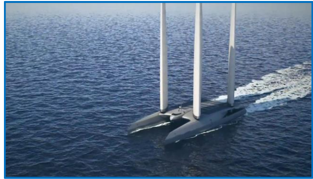
The Drift project. Rated power 1-2 MW, Length 58 meters, H 2 Production 150 t/a. Credit to https://drift.energy/ (UK).
