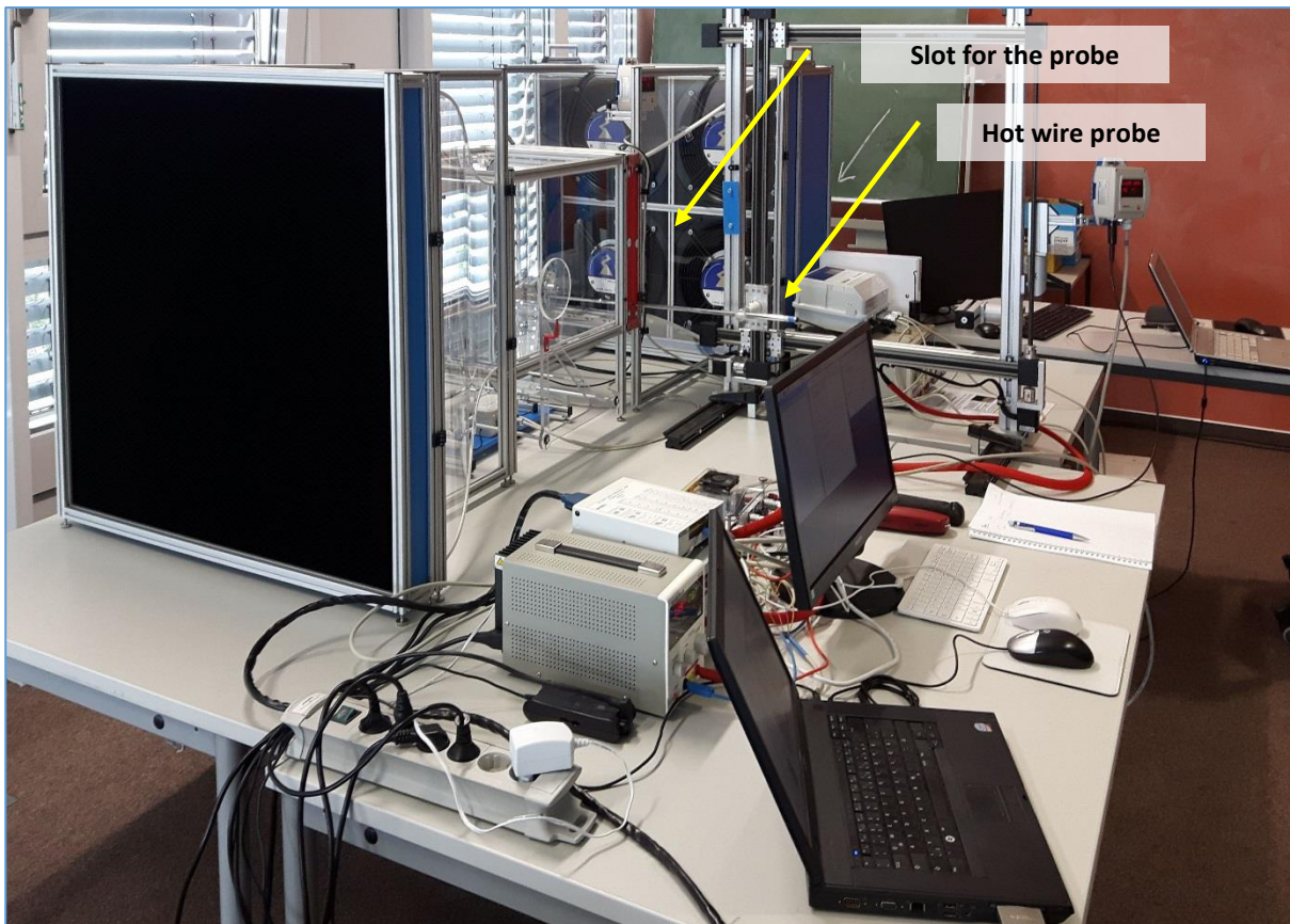
GWK3 with traversing device ANIPROP TRV1 - Existing measuring technology
