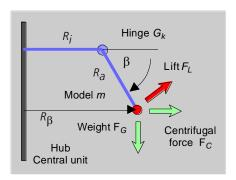
Gravity acceleration g; circular frequency  $\omega = 2 \cdot \pi / T$ , where T is the time for one rotation.
