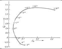
Lift and drag, respectively their coefficients, may be thought as functions depending on the angle of incidence  $\alpha$ :
