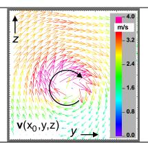
Method to visualise a velocity field, e.g. the flow around or behind a wing. A flow containing small particles (diameter d in the order of  $10^6$  m) streams around an obstacle. Two subsequent pictures of this flow are taken while illuminating the stream with two laser flashes. A computer programme tries to identify the particles in the first picture also in the second picture (i.e. finding the trace).
