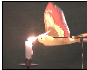
Fig. 10,11. The artificial bird shows how the air is taken in during the flapping motion.
